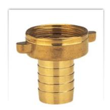
The two-piece Threaded Hose Coupling comprises a socket and sleeve nut; it is therefore a flat washer seal. It is suitable as a connection to the tap, however not for pumps. With  $33.3 \, \text{mm}$  (G 1") thread, suitable for  $25 \, \text{mm}$  (1") hoses.
